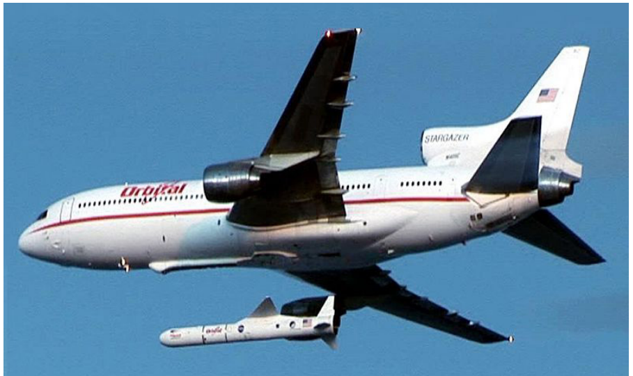
Fig. 2.1.4-1 Release of the Pegasus XL launch vehicle from its carrier aircraft.
