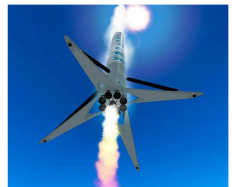
Fig. 2.1.4-3 A computer image of the descending US Falcon-9R's first stage, slowing the velocity of its decent with one of its main engines.
