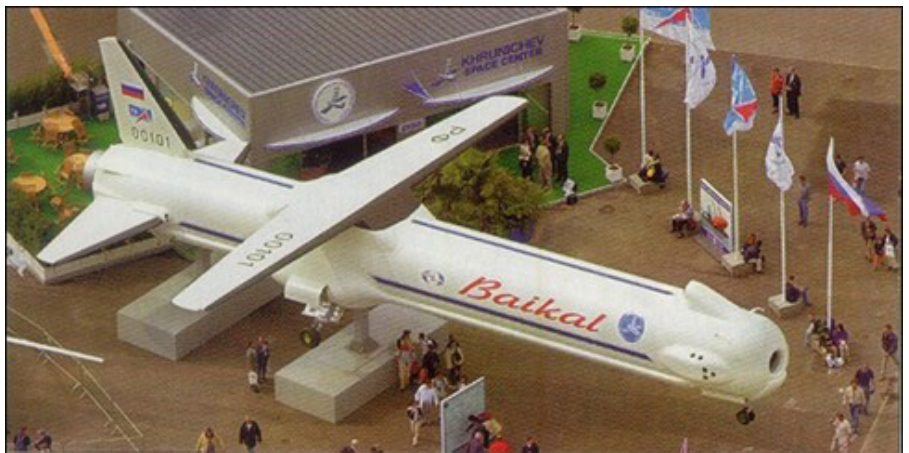
Fig. 2.1.4-2 A full-scale engineering mock-up of the Russian Baikal fly-back booster, at the Paris Airshow-2001 in Le-Bourget.
