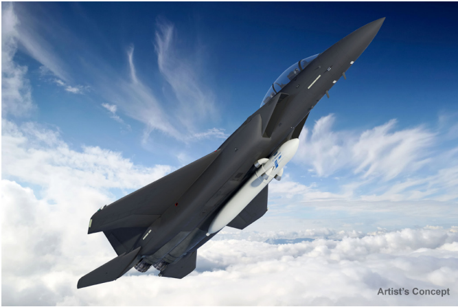
Fig. 7.1-1 Boeing's ALASA concept involves the air launch of a rocket from an F-15E
